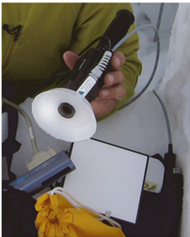
Fig. 1. Contact probe with an unpainted slip-on spacer to facilitate view of configuration. The slip-on spacer that is implemented in the field has been coated with thick, flat black paint to occlude all radiation other than that from the probe illumination.
