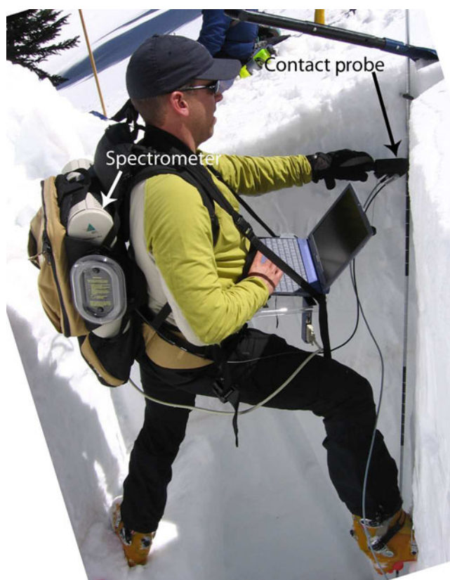
Fig. 2. Contact probe in use in the San Juan Mountains.
